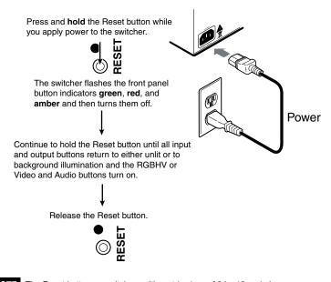
NOTE The Reset button on switchers with matrix sizes of 24 x 12 and above have a different appearance and do not have a rear panel Reset LED.
